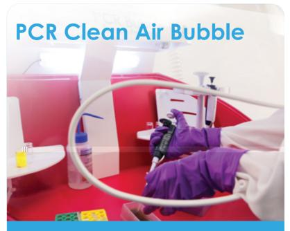
The PCR Clean Air Bubble provides a comfortable to use, easy to clean, HEPA filtered clean air environment for the preparation of PCR reagents. The integrated UV-C Germicidal Lamp provides effective biodecontamination.
